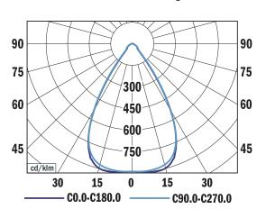
TRUXIAN M LME, 9800 lm 4000 K LOR = 100% lower flux fraction 100% upper flux fraction 0%
