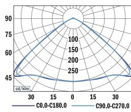
TRUXIAN M LEW, 9800 lm 4000 K LOR = 100% lower flux fraction 100% upper flux fraction 0%
