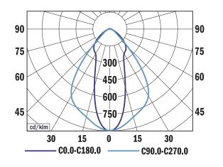
TRUXIAN M LCO, 9800 lm 4000 K LOR = 100% lower flux fraction 100% upper flux fraction 0%
