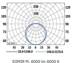
LOR = 100% lower flux fraction 93% upper flux fraction 7% UGR < 28
