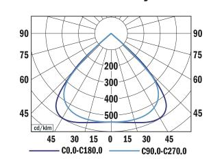
LUMIXIAN 90°, 14,700 lm 4000 K LOR = 100% lower flux fraction 100% upper flux fraction 0% UGR < 28
