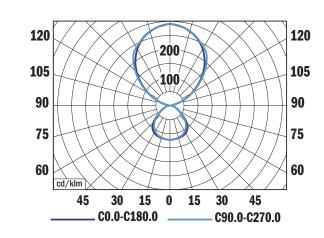
LAMBDA FREESTANDING, 7050 lm 4000 K LOR = 100% lower flux fraction 69% upper flux fraction 31% UGR < 16
