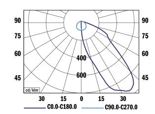
LAMBDA ASYMMETRIC M, 2450 lm 4000 K LOR = 100% lower flux fraction 100% upper flux fraction 0%
