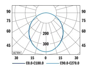
GACRUX IP54 OPD PV1, 3800 lm 4000 K LOR = 100% lower flux fraction 100% upper flux fraction 0% UGR < 22
