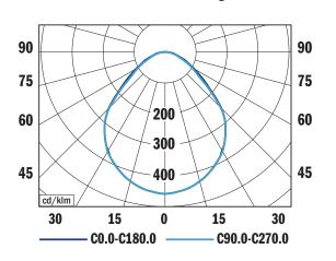
GACRUX IP54 MCD PV1, 3300 lm 4000 K LOR = 100% lower flux fraction 100% upper flux fraction 0% UGR < 19
