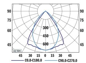
DECLAN SS1, 3800 lm 4000 K LOR = 100% lower flux fraction 100% upper flux fraction 0% UGR < 19
