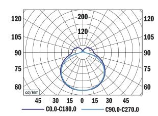
CORIS IP54 M, 4900 lm 4000 K LOR = 100% lower flux fraction 81% upper flux fraction 19% UGR < 25
