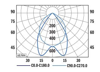
CLASSIC M, 4500 lm 4000 K LOR = 100% lower flux fraction 100% upper flux fraction 0% UGR <16/<19
