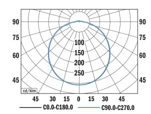
BANOR IP54 S, 1700 lm 4000 K LOR = 100% lower flux fraction 96% upper flux fraction 4% UGR < 28
