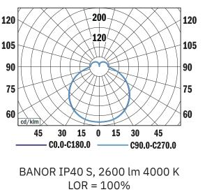
lower flux fraction 81% upper flux fraction 19% UGR < 25
