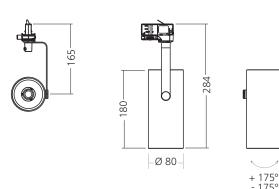
1400 lm, 1300 lm, 2250 lm, 2350 lm (CADAN/CADAN S) 2400 lm, 2550 lm, 4100 lm, 4350 lm (CADAN IB) 10 W, 17 W (CADAN/CADAN S) 21 W, 36 W (CADAN IB) 114-140 lm/W 3-step MacAdam > 80 3000 K, 4000 K FIX Facet reflector 24°, 40° Housing: extruded aluminium Reflector: facet anodised aluminium Black RAL 9005 100,000 hours/L90/B50 From -25 °C to +35 °C
