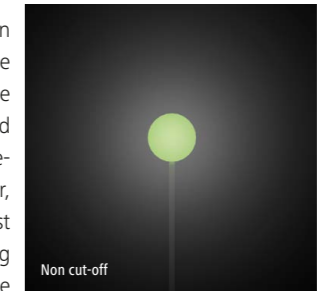
A Generally pole mounted luminaires with a globe shaped top that emits light in all directions. They create a lot of light pollution and are very glaring. They are rarely used on roads but are still often found in residential and urban areas.
