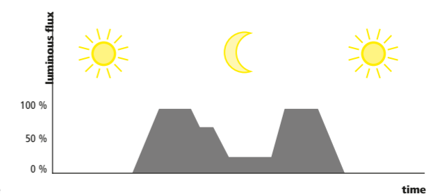
C Single phase switching with twilight sensor.
