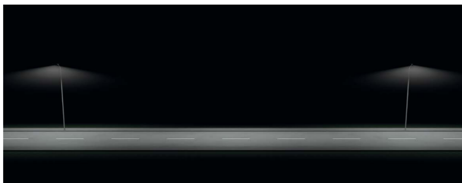
D Luminaires with high performance optics that emit light laterally over a large distance, ensuring that the road is evenly illuminated, and visual acuity maintained.
