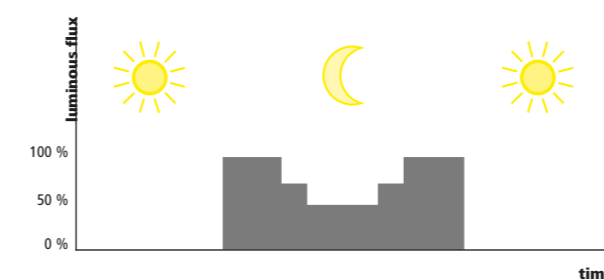
B Single phase switching with twilight sensor.
