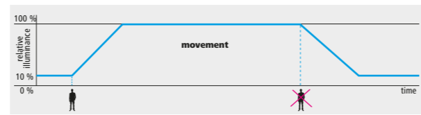
Time procedure of presence detector - without delay
