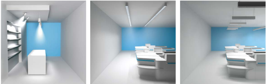
A boutique style payment counter using statement suspended luminaires to highlight and illuminate the counter, and accent lighting spotlights to provide suitable vertical illumination of the display behind. In larger stores such as supermarkets where check-outs are located next to each other, it is beneficial to use continuous line lighting to ensure sufficient levels of illumination with minimal glare.
