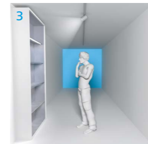
3 By positioning LED strip luminaires on the lower edge of shelves, all shelves are optimally illuminated. LED light sources are perfect for this because they emit negligible amounts of heat, allowing them to be positioned very close to even fragile items.
