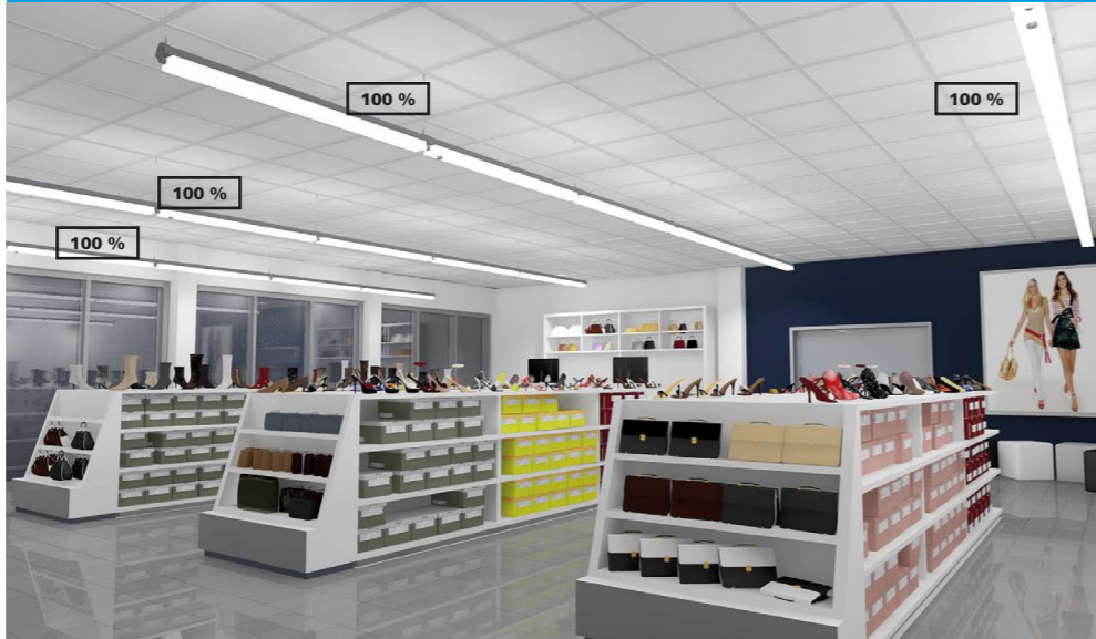
If there is not sufficient daylight available (such as during evening hours) all luminaires automatically work at full luminous flux.
