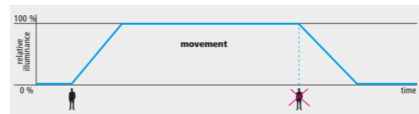
Time procedure of presence detector - without delay
