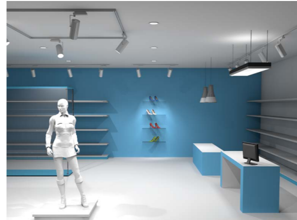
Morning lighting scene: Payment counter 100 %, promotion display lighting 100 %, accent lighting 100 %, general lighting 100 %. All lighting elements function at 100 % luminous output. The brightness is activating and stimulating to customers who are only just starting their day.
