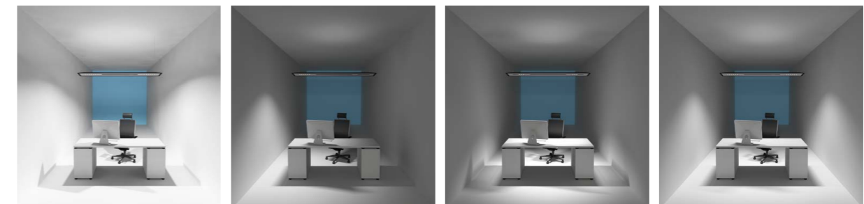
The LED sources with various luminous intensity which reflect the light from the built-in reflectors under different angles enable changing the width of the luminous intensity curve within one luminaire.
