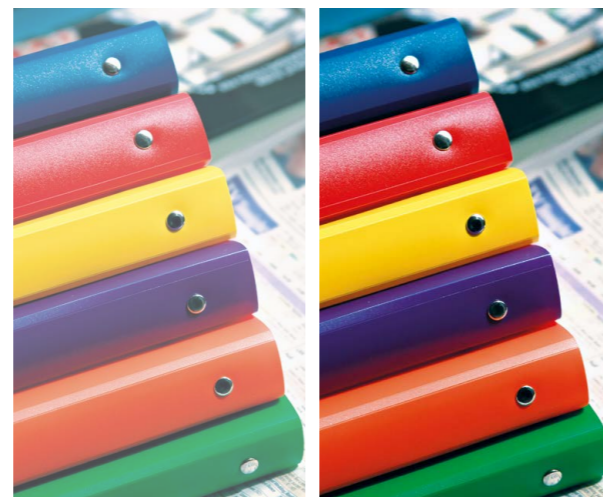
Comparison of colour rendering indexes – CRI. Left: CRI 70. Right: CRI 93
