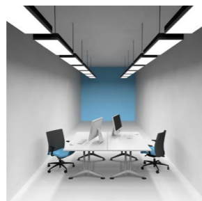
Luminaires with direct characteristic of the luminous flow distribution are insufficient for the harmonious distribution of brightness in the office.
