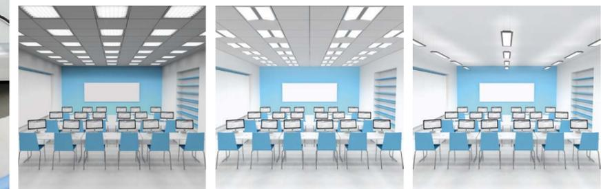
The recessed luminaires with louvers – see the figure 1 – do not provide sufficient illuminance of the vertical surfaces and ceiling. At the same time they represent a risk of arising undesirable reflections on the screens due to the indirect glare. The recessed or suspended luminaires with the direct and indirect characteristic of radiation with diffuse surface or microprism represent an optimal solution.
