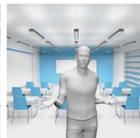
For the correct modelling of the faces it is important to ensure in the classrooms sufficient cylindrical illuminance amounting 150 lux. The suspended luminaires with the direct and indirect characteristic of the luminous flux distribution which eliminate forming undesirable shadows and at the same time do not cause glare are the optimal solution.
