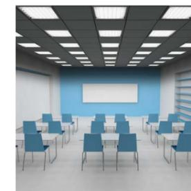
*The recessed luminaires with louver with the direct characteristic of the luminous flux distribution are not suitable for the classrooms. We will not achieve the sufficient illuminance of the ceiling.*
