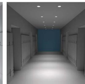
The presence detector can be adjusted in such a way that the lighting in an abandoned space will not switch off immediately after departure of the last person but gradually.
