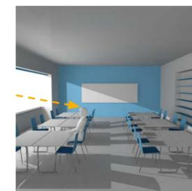
Direct glare can be prevented by correct organisation of the working plane. Placing the desks rectangular to the windows will prevent pupils to be directly exposed to the sunshine and thus to the undesirable glare.
