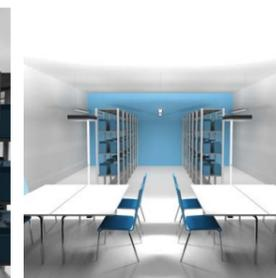
When designing the library lighting system the emphasis is laid also on the vertical illumination of the racks and shelves. The correctly illuminated racks ensure sufficient visibility of the books from the highest shelf to bottom one. The linear suspended luminaires with the direct and indirect radiation component, located along the aisles between individual book shelves are considered a suitable solution. The standard EN 12464-1 determines the minimal illuminance 200 lux for the racks.
