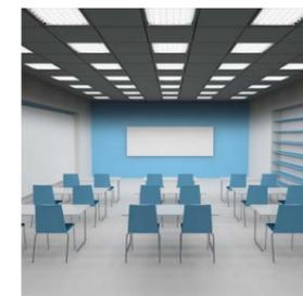
The classical solution of the classroom lighting with recessed luminaires with a parabolic louvre ensures sufficient illumination of the workplace but the upper parts of the walls and the ceiling remain dark. Such illumination causes a feeling of a cave effect and makes the classroom optically smaller.
