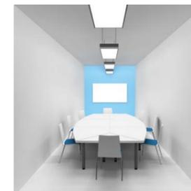
Optimal lighting solution in this space is represented by suspension luminaires with direct and indirect characteristics of the luminous flux distribution. The indirect diffuse light helps to model objects, it reduces indirect glare when the light reflects from the PC screen or the shiny surfaces in the room.
