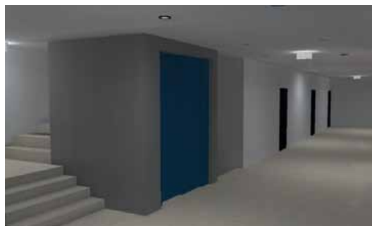
The final DIALux output shows the expected lighting conditions provided by the emergency lighting system in the case of a power failure.
