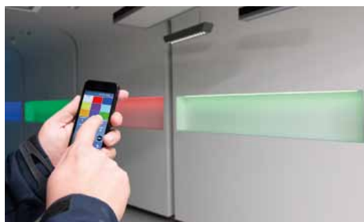
The GUI allows for the increases and decreasing of illumination level, or the change of light colour according to desire or need.
