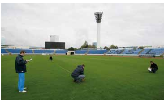
Before the illumination can be directed the calculation of suitable measuring points must be performed.
