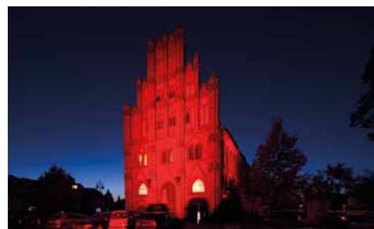
The original illumination of the facade did not draw deserved attention to the architecture. The new RGB colour mixing solution emphasises the cultural and spiritual soul of the building.
