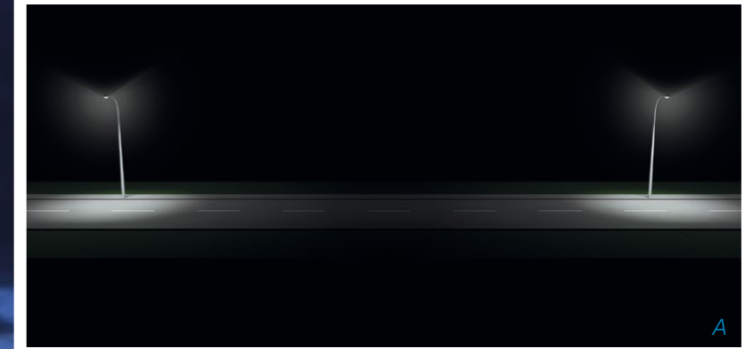
Figure 19A An installation using conventional luminaires that illuminate unevenly, creating 'hot spots' that reduce visual acuity
