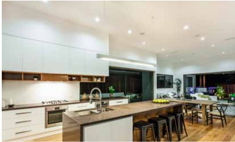
Figure 17 Use general lighting to facilitate visual acuity by effectively illuminating surfaces such as table tops, kitchen counters and desks to enable the performance of tasks, as well as floors to aid navigation.
