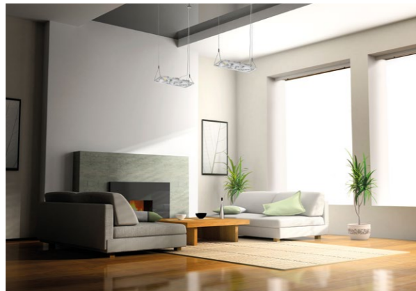
Uncontrolled sunlight causes areas of extreme brightness that contrasts against areas with much lower luminance levels. This results in visual discomfort and reduced perception. Often, people will turn the lighting on to try and balance the difference.
