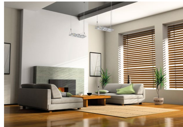
Solar shading distributes the light entering the room more evenly, minimising differences between brighter and darker areas. If the resultant overall light level is sufficient it is not necessary to turn any artificial lighting on at all.
