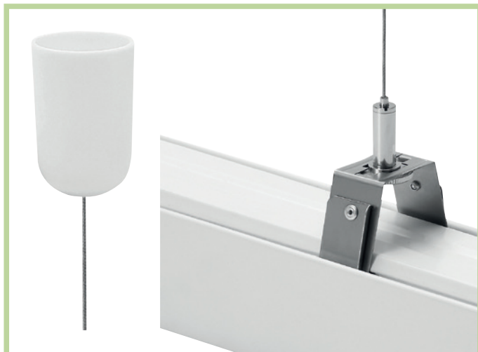
RS 02 suspension An adjustable 1.5 mm diameter rope is used for the suspension of mounting rails. Standardly supplied with a length of 1000 mm, other lengths are available on request.
