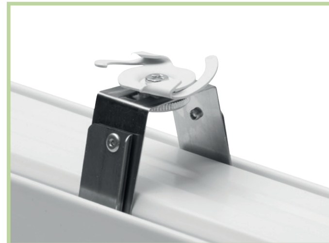
SB 02 T24 bracket for ceiling mounting A quick-fix bracket for mounting of the mounting rails in T-profile (24 mm) ceilings.
