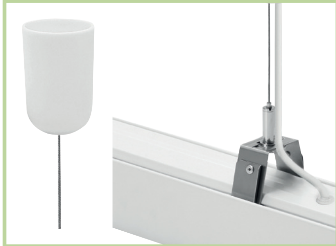
RSE 02 suspension with electric cable An adjustable rope is used for the suspension of the mounting rail along with cables for connection to the mains. Cables are standardly supplied with a length of 1000 mm.
